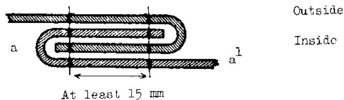
\*/ Threads visible from the inside shall be of a colour different from that of the threads visible from the outside and from that of the sheet.
